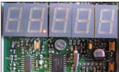
5-figure display, with 4 push buttons
